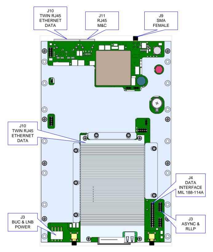
Figure 4-4. Baseband Modem Board (PL-0021833)
