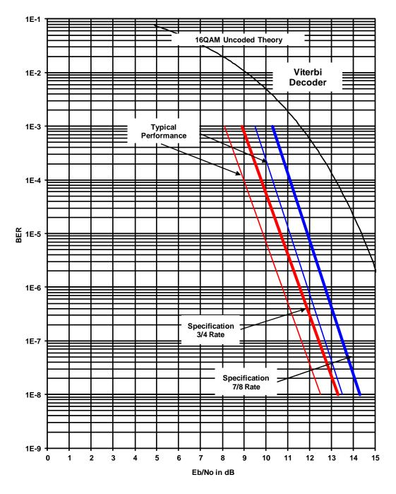
Figure 6-5. DMD1050T 16QAM BER Performance (Viterbi)
