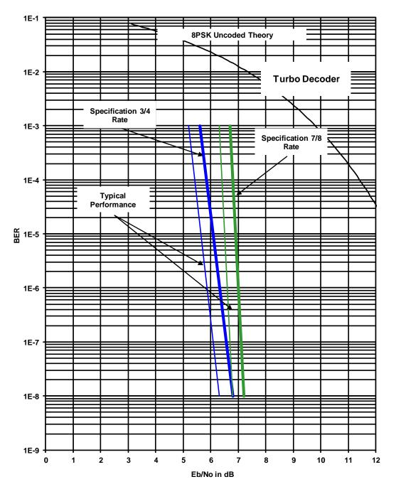
Figure 6-9. DMD1050T 8PSK BER Performance (Turbo)
