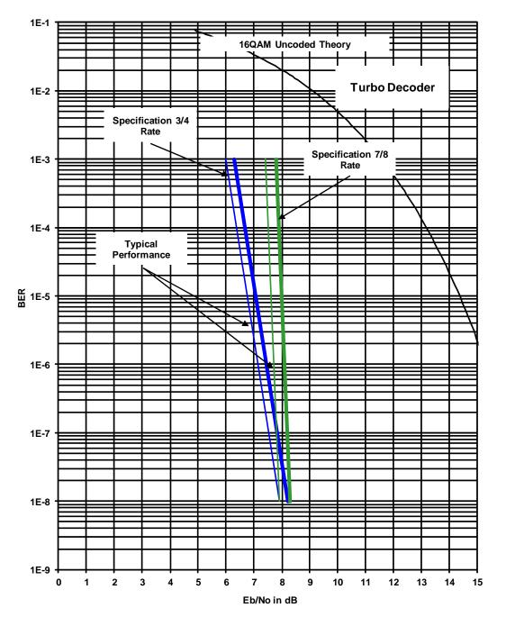
Figure 6-10. DMD1050T 16QAM BER Performance (Turbo)
