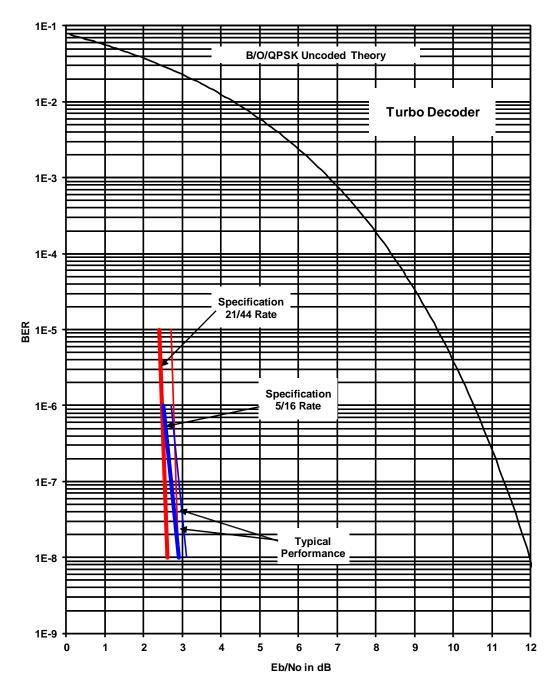
Figure 6-8. DMD1050T BPSK BER Performance (Turbo)
