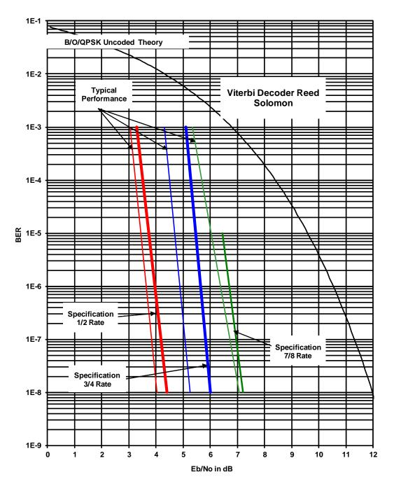
Figure 6-3. DMD1050T B/O/QPSK BER Performance (Viterbi – w/RS)
