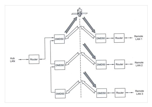
Figure 3-6 Point-to-Multipoint with Daisy Chaining
