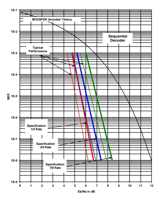
Figure 6-2. DMD1050T B/0/QPSK BER Performance (Sequential)
