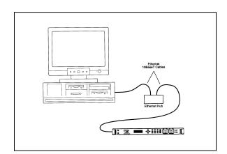
Figure D-1 Ethernet Connection
