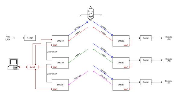
Figure F-6 Remote Monitor and Control
