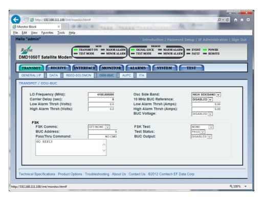
Figure 7-15 Transmit / ODU-BUC Menu
