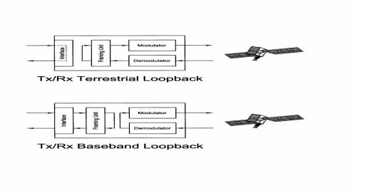
Figure 3-9 Loopback Functional Block Diagram
