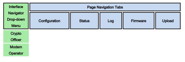
The **Interface Navigator Drop-down Menu** and its selections (shown in green) allow secure access to one of the DMD1050T's three, distinct Web interfaces.
