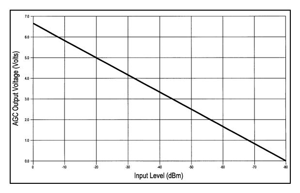
Figure 6-14. AGC Voltage Monitor
