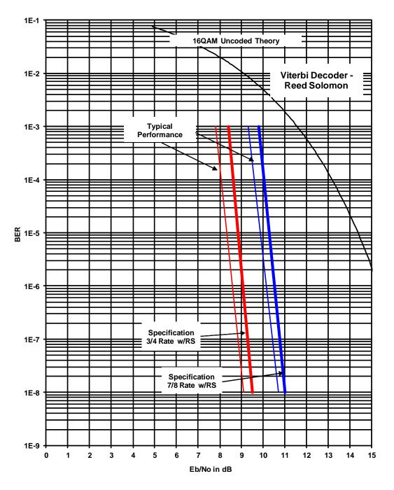
Figure 6-6. DMD1050T 16QAM BER Performance (Viterbi w/RS)
