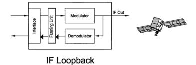
Figure 3-8 Loopback Functional Block Diagram
