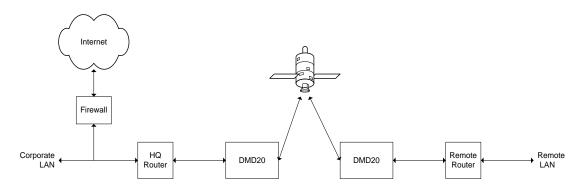
Figure F-1 Point-to-Point Applications
