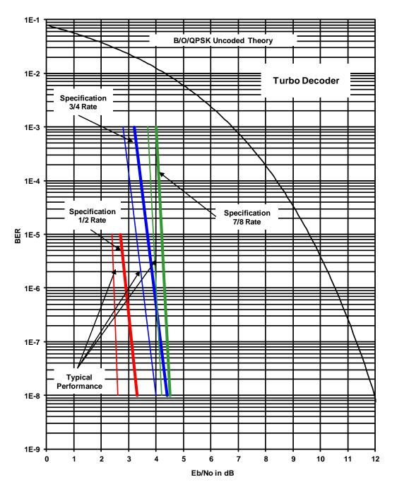
Figure 6-7. DMD1050T (O)QPSK BER Performance (Turbo)
