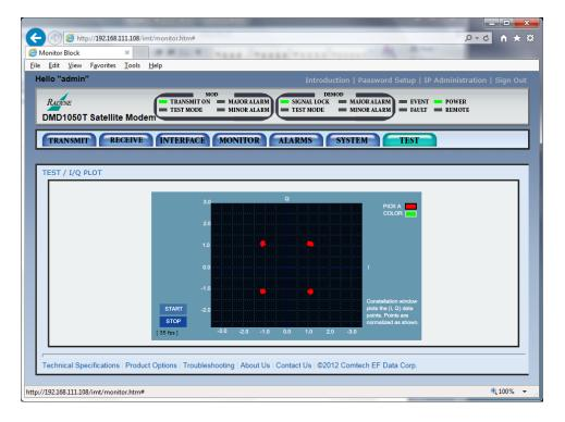
Figure 7-35 Test / IQ Plot page example
